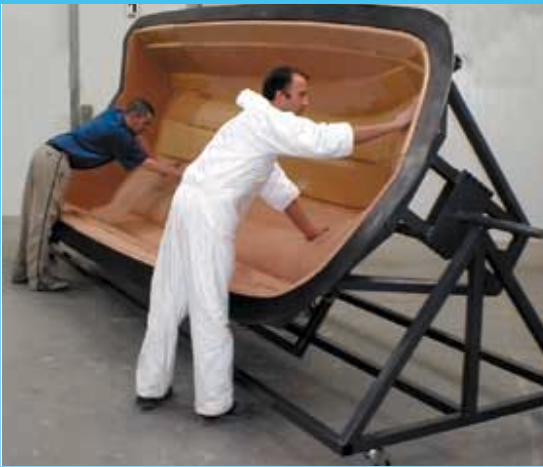
Gimbed face mould is calibrated in readiness for second mould half manufacture
