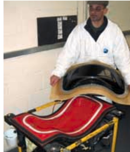
Temperature controlled LRTM carbon fibre wing mould
