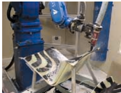
Mouldings trimmed by robot
