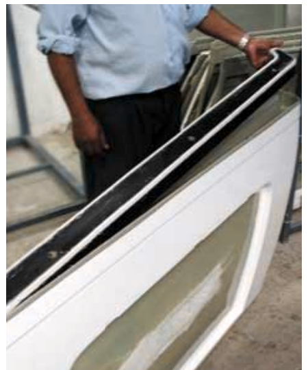
Lower side action tool extraction from part
