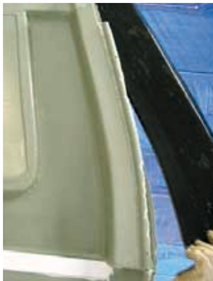
Rear side action tool extraction from part
