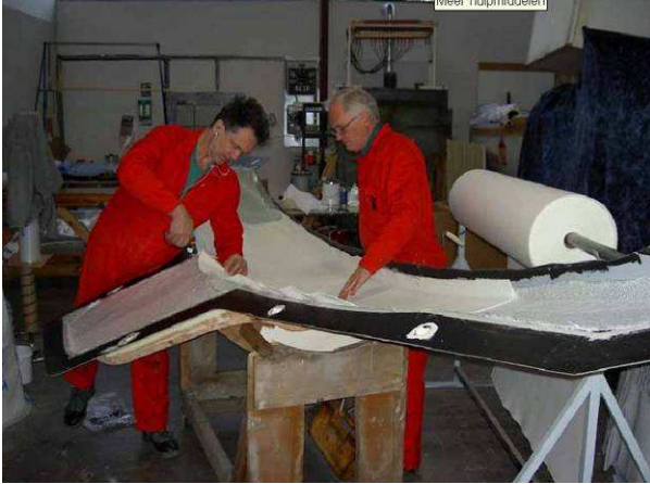
Figure 10: Malmsten Boats (S) application of Soric in a small hull of a sail boat.
