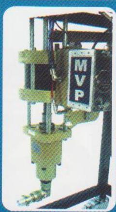
Ideal freedom for maintenance provided by unlocking and rapid removal of the entire Patriot pump assembly in seconds. The Patriot pump system, as a whole, can be unlocked and removed as one complete unit without the use of tools allowing it to be brought to bench working height. This feature enables the user to carry out routine maintenance in ideal and accessible conditions
