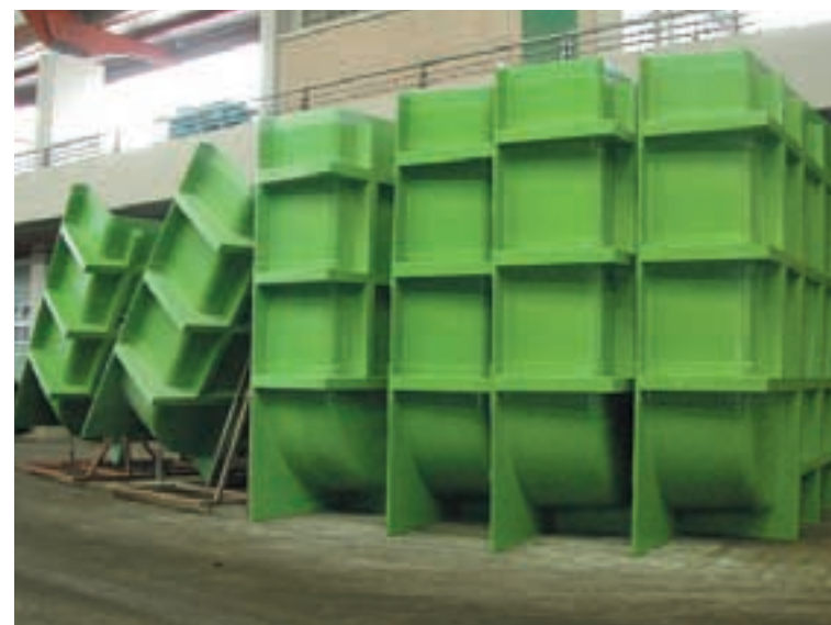
Finished tank sections ready for installation
