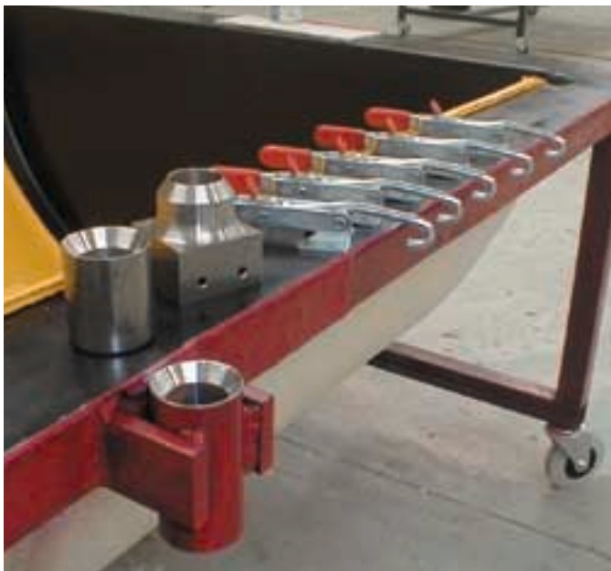
One M24 clamp/dowel station replaces at least 5 latch clamps
