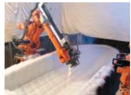
RIMFIRE™ control software delivers accurate placement of glass preform.
