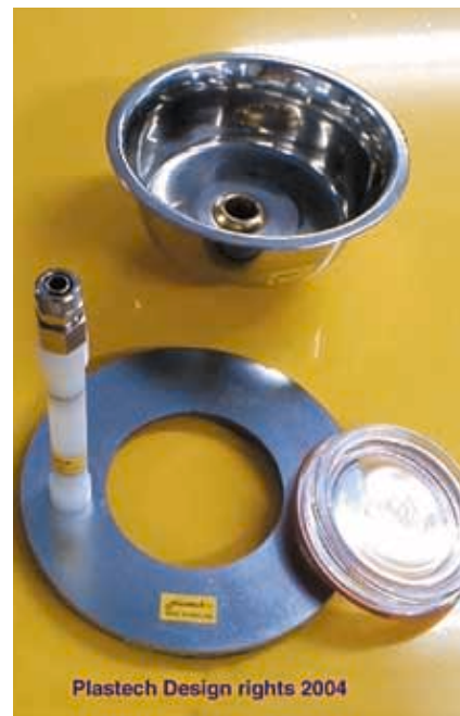
New catchpot fitted with removable sealed window and resin arrestor
