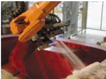
Robotic arm carries high output RIMFIRE™ fibre/binder dispense head
