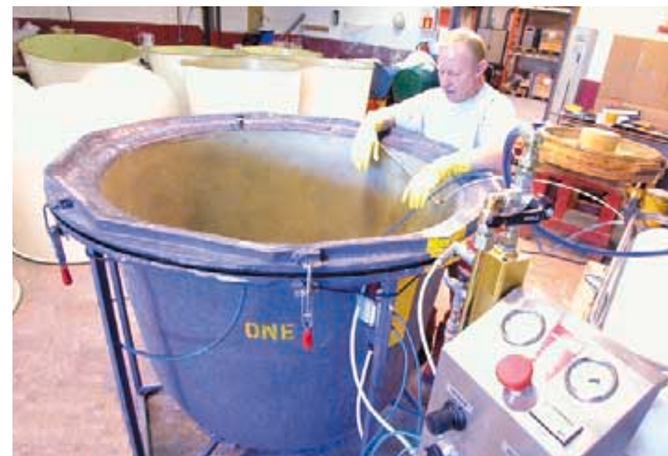
5m 2 Light RTM Radome production at Biobe
