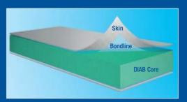
The DIAB sandwich concept increases structural performance while optimizing weight. A sandwich consists of two high strength skins or facings separated by a core material. The skins take up the bending stresses and give the structure a hard wearing surface. The light DIAB core absorbs the shear stresses and distributes them over a larger area.
