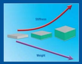
Compared to monolithic composite laminates or metals, the sandwich concept significantly reduces weight and increases stiffness while maintaining strength. Even higher strength and stiffness properties can be achieved by increasing the thickness of the core without a weight penalty.
